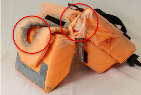
Discoloured and torn foam life jacket
