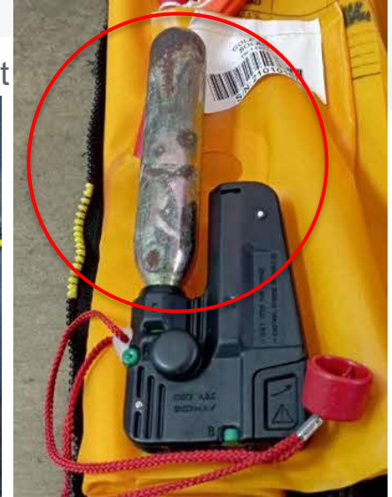
Corroded gas cartridge
